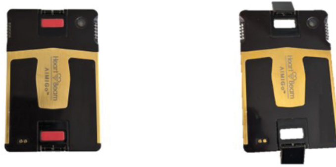
Photographs of Version 1 AIMIGo devices in planar and ready to use position.
