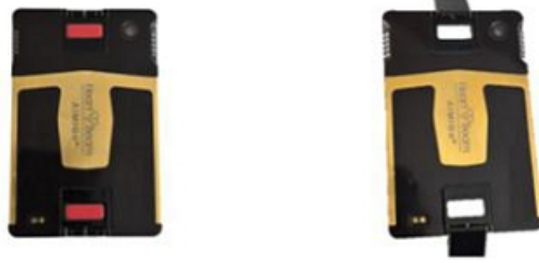
Photographs of version 1 HeartBeam AIMiGo devices in planer and ready to use position.
